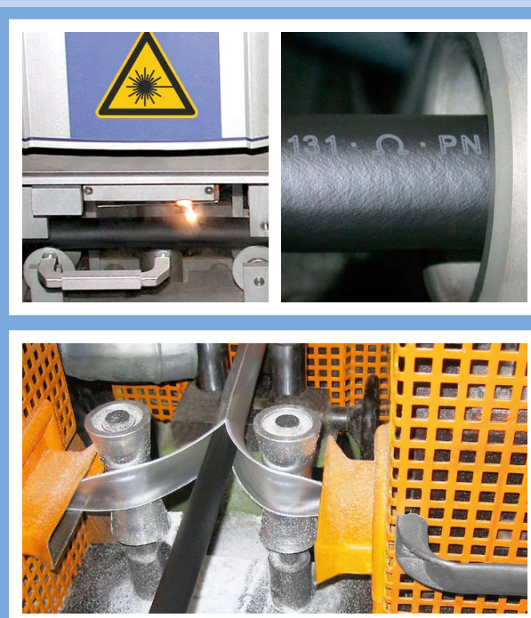
Continuous laser marking · Peeling off the plastic cover after vulcanisation
