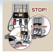
Filling is instantly stopped when the Impact detection sensor senses acceleration by the accident or earthquake.
